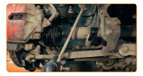
Replacement: anti roll bar links – VW Beetle Convertible (5C7, 5C8). Tip from AUTODOC experts:
