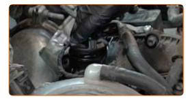
Tighten the oil filler cap.
