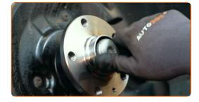
Tighten the fastener of the wheel hub bearing. Use XZN #18. Use a torque wrench. Tighten it to 200 Nm torque.
