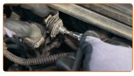
6 Unscrew the brake fluid reservoir cap.
