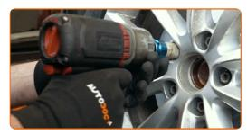
Lower the car and working in a cross order, tighten the wheel bolts. Use wheel impact socket #17. Use a torque 21 wrench. Tighten it to 120 Nm torque.
