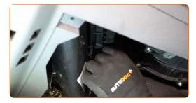
Screw in the fasteners of the cabin filter housing cover. Use a drive socket #5,5. Use a ratchet wrench.
