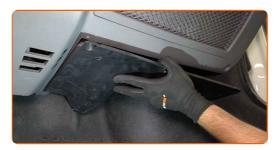
Screw in the fasteners of the passenger side kick panel. Use Torx T20.
