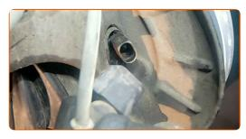
Clean the ABS sensor fastener. Use a wire brush. Use WD-40 spray.
