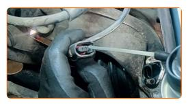
15 Attach the ABS sensor connector.
