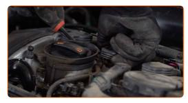
Take out the ignition coils from the spark plug wells.
