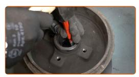
Install the new inner race of the wheel bearing into the brake drum. Use a bush and bearing driver set. Use a hammer.
