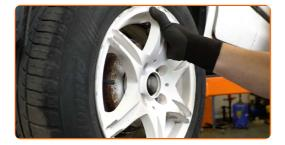
Remove the wheel hub nut cap. Use a crowbar. Use a hammer.
