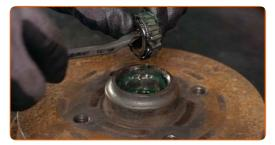
Remove the inner oil seal of the wheel bearing. Use a crowbar.
