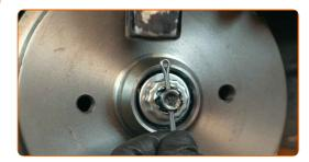
Install the cap of the hub nut. Use a hammer.
