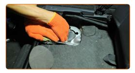
17 Remove the protective cap of the shock absorber mount.
