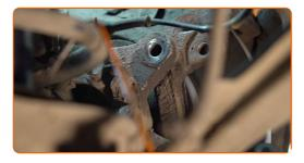
Tighten the brake caliper bracket. Use a combination spanner #13. Use a torque wrench. Tighten it to 35 Nm torque.+60°
