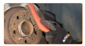
Unscrew the brake disc fastening. Use a drive socket #10. Use a ratchet wrench.
