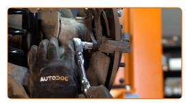
Remove the caliper bracket.
