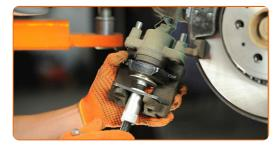
Install the brake caliper and fix it. Use HEX No.H7. Use a torque wrench. Tighten it to 28 Nm torque.
