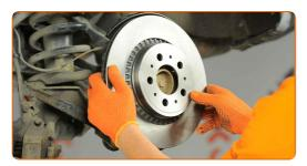
Tighten the brake disc fastening. Use a drive socket #10. Use a torque wrench. Tighten it to 11 Nm torque.
