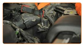
6 Slightly raise the cover of the air filter housing.
