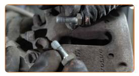
12 Remove the brake caliper.
