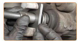
Treat the brake pads in the area where their surface comes into contact with the brake caliper bracket. Use antisqueal paste.
