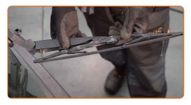
Remove the blade from the wiper arm.
