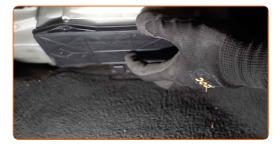
Screw in the fasteners of the cabin filter housing cover. Use Torx T20. Use a ratchet wrench.
