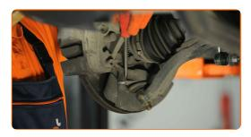
Disconnect the spherical joint from the arm. Use a ball joint puller.
