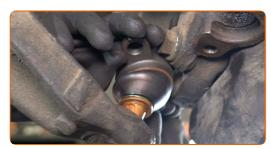
Connect the ball joint to the steering knuckle. Use a crowbar. Use a rubber mallet.
