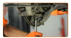
Tighten the fasteners connecting the ball joint to the control arm. Use a drive socket #21. Use a torque wrench. Tighten it to 100 nm torque.
