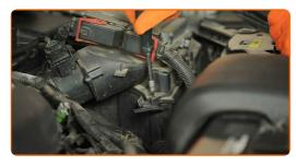
6 Slightly raise the cover of the air filter housing.
