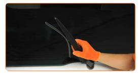
Remove the blade from the wiper arm.
