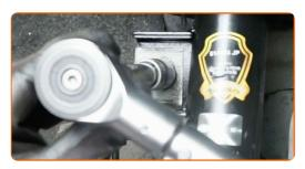
Tighten the fastening nut connecting the tie rod end to the steering knuckle. Use a drive socket #22. Use a torque wrench. Tighten it to 80 Nm torque.
