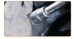
Tighten the fastener connecting the ball joint to the steering knuckle. Use a combination spanner #21. Use a torque wrench. Tighten it to 110 Nm torque.
