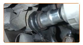
Attach the brake hose to the suspension strut.
