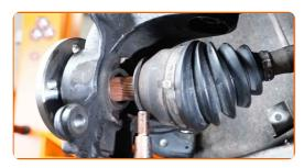
Connect the ball joint to the steering knuckle. Use a crowbar.
