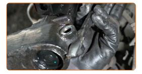
Disconnect the steering knuckle from the suspension strut. Use a rubber mallet.
