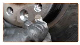
18 Remove the brake disc.
