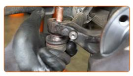
Screw on the fastening nut that connects the tie rod end to the steering knuckle. Use a drive socket #22. Use a ratchet wrench.
