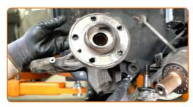
Clean the suspension strut mounting seat on the steering knuckle. Use a wire brush.
