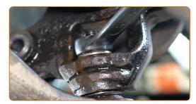
Disconnect the ball joint from the steering knuckle. Use a ball joint puller. Use a crowbar.
