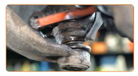
Unscrew the fastener connecting the ball joint to the steering knuckle. Use a combination spanner #21.
