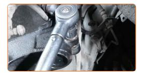
Tighten the brake caliper bracket fasteners. Use a drive socket #18. Use a torque wrench. Tighten it to 150 Nm torque.
