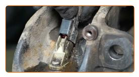
Disconnect the ABS sensor wiring.
