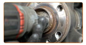
Remove the fastening bolt.
