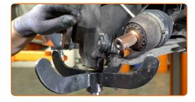
Release the lower fastener connecting the shock strut to the steering knuckle. Use a flat metal-working chisel. Use a hammer.
