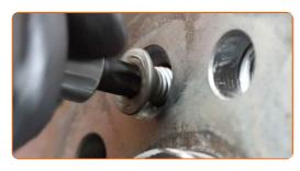
75 Tighten the brake disc fasteners. Use Torx T50. Use a torque wrench. Tighten it to 15 Nm torque.
