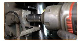
Disconnect the sway bar link from the suspension strut.
