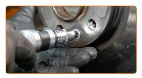
17 Remove the fastening bolt.
