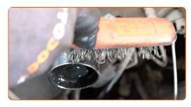
Clean the fastener that connects the sway bar link to the suspension strut. Use a wire brush.
