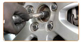
Loosen the wheel bolts. Use wheel impact socket #19. Use a tap wrench.
