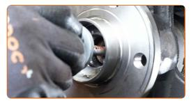
Screw in the fastener of the CV axle. Use a drive socket #13. Use a ratchet wrench.
