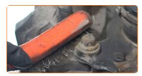
Unscrew the brake caliper bracket fasteners. Use a drive socket #18. Use a ratchet wrench.
