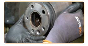
Unscrew the fastener connecting the drive shaft to the wheel hub. Use a drive socket #13. Use a ratchet wrench.
