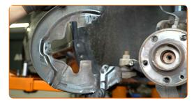
Clean the ABS sensor connector. Use a nylon cleaning brush. Use all-purpose cleaning spray.
