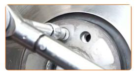
76 Install the brake caliper together with its bracket.
