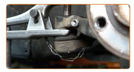
Clean the lower fastener connecting the suspension strut to the steering knuckle. Use a wire brush. Use WD-40 spray.
