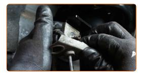
Screw in the fastener connecting the sway bar link to the suspension strut. Use a drive socket #15. Use a ratchet wrench.
