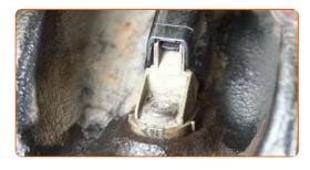
69 Install the brake disc cover.
