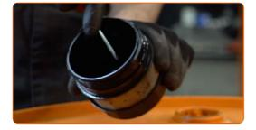
Install a new O-ring to its mounting seat on the filter cover.
