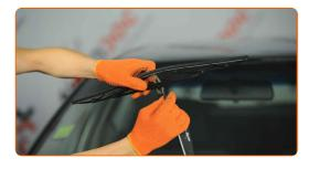
Remove the blade from the wiper arm.
