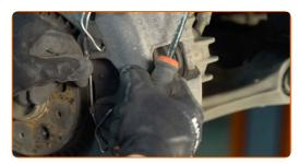
11 Remove the brake caliper.
