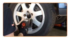
Lower the car and working in a cross order, tighten the wheel bolts. Use wheel impact socket #19. Use a torque wrench. Tighten it to 140 nm torque.
