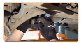
Tighten the fastener connecting the stabilizer link to the stabilizer bar. Use a combination spanner #18. Use a drive socket #18. Use a torque wrench. Tighten it to 60 Nm torque.
