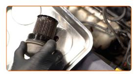
Replacement: engine oil and filter – VOLVO V40 Hatchback (525, 526). Tip from AUTODOC experts:
