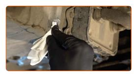
Screw in the new drainage plug and tighten it. Use a drive socket #15. Use a torque wrench. Tighten it to 38 nm torque.
