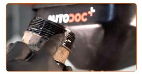
Screw the new filter into its place. Use the 86/14-F socket. Use a torque wrench. Tighten it to 25 nm torque.
