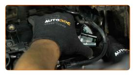
Screw the fixing bolts of the fuel filter bracket. Use a drive socket #8. Use a ratchet wrench.
