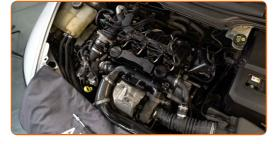
Unscrew the fuel filter bracket fixing bolts. Use a drive socket #8. Use a drive socket #10. Use a ratchet wrench.
