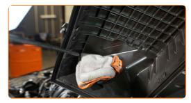
9 Insert a new filter element into the filter housing.
