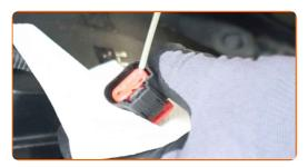
Attach the mass air flow sensor connector.
