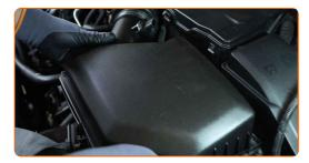
Screw in the fastening screws of the air filter cover. Use Torx T25. Use a ratchet wrench.
