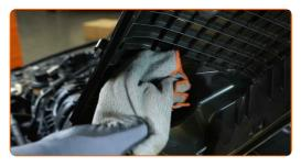
Install the air filter cover. Fasten it.
