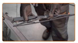
Remove the blade from the wiper arm.
