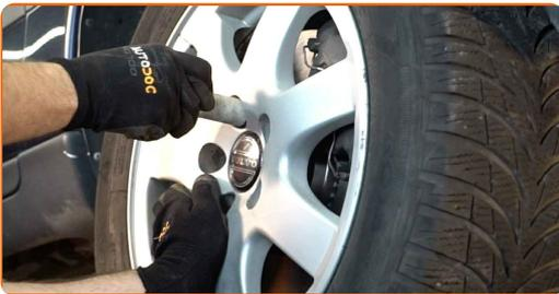
**57** Lower the car and working in a cross order, tighten the wheel bolts. Use a torque wrench. Tighten it to 140 Nm torque.
