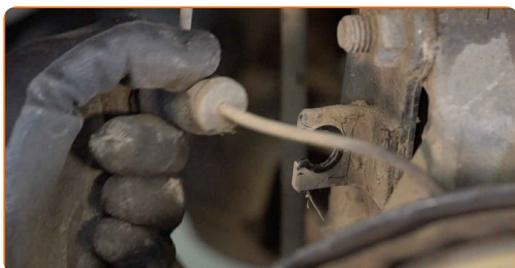
**13** Clean the fasteners connecting the shock strut to the steering knuckle. Use a wire brush. Use WD-40 spray.
