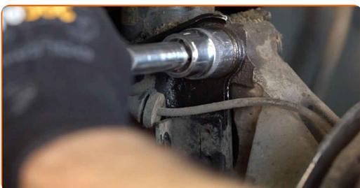
**15** Prop up the steering knuckle. Use a hydraulic transmission jack.
