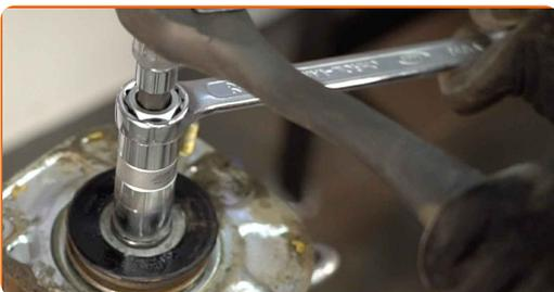
**25** Unscrew the fastener of the shock strut mount. Use HEX No.H6. Use a ratchet wrench. Use water pump pliers.
