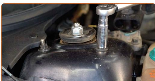
**51** Treat the shock strut fasteners. Treat the shock strut rod. Use copper grease.
