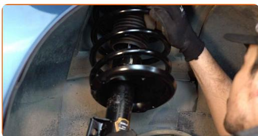
**39** Screw the top fastening of the shock strut mount. Do not tighten it.
