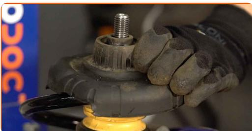
**34** Screw in the fastener of the shock strut mount. Use HEX No.H6. Use a ratchet wrench. Use water pump pliers.
