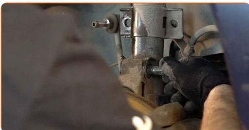
**17** Disconnect the steering knuckle from the shock absorber strut.
