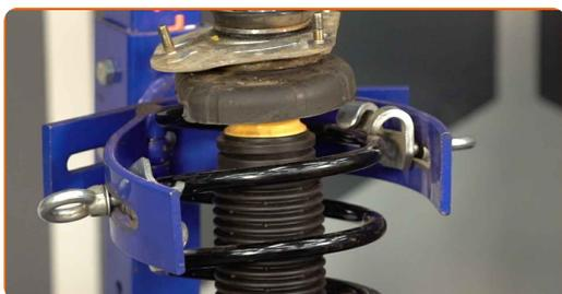
**37** Remove the assembled shock strut.
