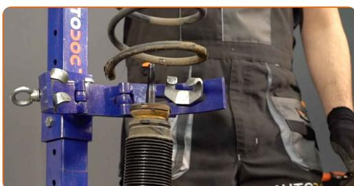
**29** Remove the shock absorber dust cap and the bump stop.
