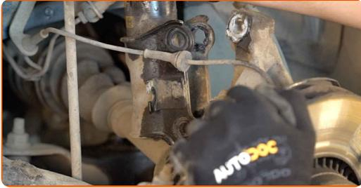
**18** Unscrew the top fastening of the shock strut mount.
