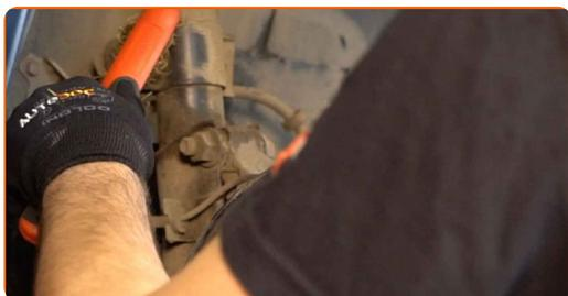
**11** Unscrew the nut and remove the stabilizer rod from the shock strut. Use a drive socket #18. Use a ratchet wrench.
