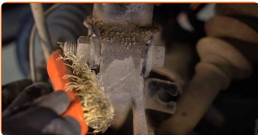
**14** Unscrew the lower fastener connecting the shock strut to the steering knuckle. Use a combination spanner #18. Use a drive socket #21. Use a ratchet wrench. Use a tap wrench.
