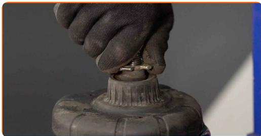
**35** Tighten the shock strut piston rod nut. Use HEX No.H6. Use a drive socket #21. Use a torque wrench. Tighten it to 65 Nm torque.
