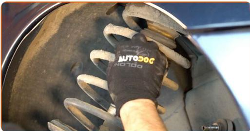
**20** Set the shock absorber strut on the spring compressor tool.
