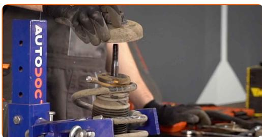
**27** Release the coil spring.
