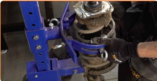
22 Remove the shock strut mount cap. Use a crowbar.
