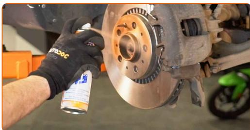
**54** Clean the brake disk surface. Use a brake cleaner.
