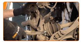
Tighten the brake caliper bracket. Use a drive socket #15. Use a torque wrench. Tighten it to 100 Nm torque.
