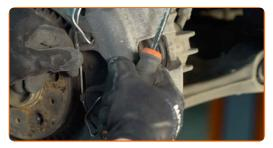
11 Remove the brake caliper.
