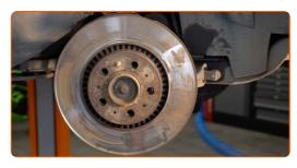
Clean the brake disk surface. Use a wire brush. Use WD-40 spray.
