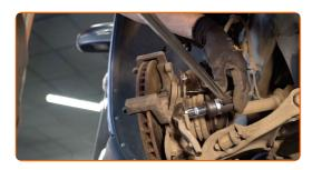
Remove the caliper bracket.
