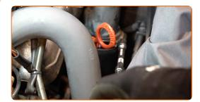
Screw in the fastener of the air intake pipe. Use a drive socket #10. Use a ratchet wrench.
