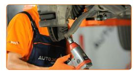
Unscrew the ball joint fastening to the steering knuckle. Use a drive socket #13. Use a ratchet wrench.
