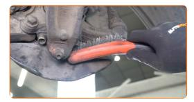
Unscrew the fastener connecting the ball joint to the suspension control arm. Use a drive socket #21. Use a ratchet wrench.
