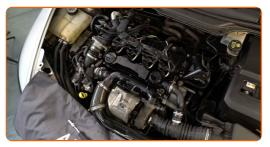
Unscrew the fuel filter bracket fixing bolts. Use a drive socket #8. Use a drive socket #10. Use a ratchet wrench.
