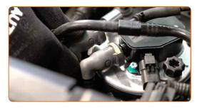
Screw the fixing bolts of the fuel filter bracket. Use a drive socket #8. Use a drive socket #10. Use a ratchet wrench.
