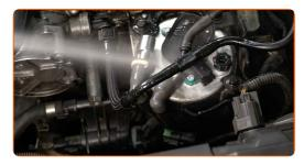
Squeeze the clips and detach the fuel supply lines from the fuel filter housing.
