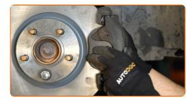
Install the brake caliper retaining spring.
