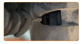
11 Remove the brake caliper.
