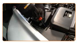
Unplug the mass air flow sensor connector.
