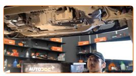
Unscrew the drain plug. Use a combination spanner #15. Use a drive socket #15. Use a ratchet wrench.
