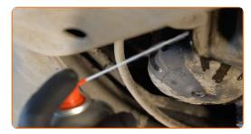
Unscrew the oil filter. Use the 86/14-F socket.
