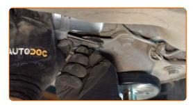
Screw the fixing bolts of the fuel filter bracket. Use a drive socket #12. Use a ratchet wrench.
