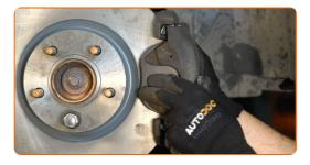
18 Install the brake caliper retaining spring.
