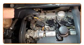
Disconnect the air intake pipe fastening. Use a drive socket #10. Use a ratchet wrench.
