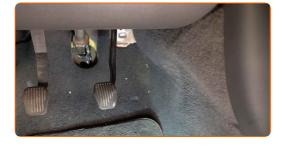
Attach the accelerator pedal connector.
