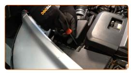
Unplug the mass air flow sensor connector.
