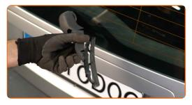
Remove the blade from the wiper arm.
