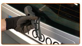
Remove the blade from the wiper arm.
