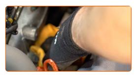
Unscrew the ignition coil bracket. Use a drive socket #10.
