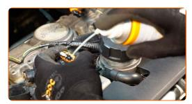
Plug in the connectors of the ignition coils. Make sure you hear a click indicating that it is locked in place.
