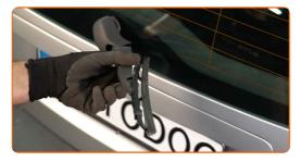
Remove the blade from the wiper arm.
