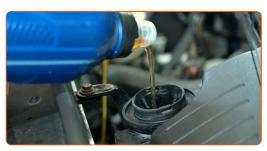
Replacement: engine oil and filter – Opel Vivaro A van. Tip from AUTODOC:
