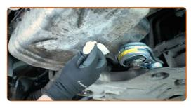
Screw in the drain plug and tighten it. Use an 8 mm square head drain plug socket. Use a torque wrench. Tightening torque: 20 N·m.
