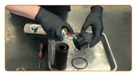
Install a new 0-ring on the oil filter cap. Install a new filter element into the oil filter cap.
