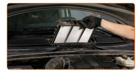
Install the cabin filter bracket. Use Torx T25. Use a torque wrench. Tighten it to 11 Nm torque.
