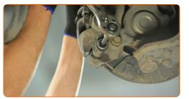
11 12 Remove the guide pins from the brake caliper.
