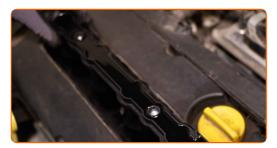
Tighten the ignition coil bolts. Use Torx T40. Use a torque wrench. Tighten it to 7 nm torque.
