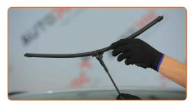
Remove the blade from the wiper arm.
